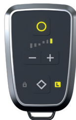
80% Throttle pedal position (Bar on right lights up)
